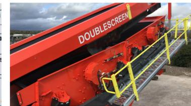
Hydraulically folding walkways for ease of maintenance
