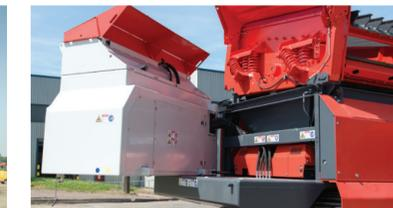
Hydraulically opening powerpack for ease of maintenance
