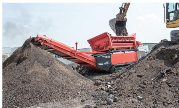
Proven, high performing heavy duty double deck vibrating grid.
