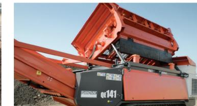
Tipping function activated by radio remote control
