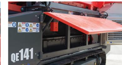
Hydraulically folding doors for easy access
