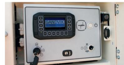
Simplified control panel for ease of operation
