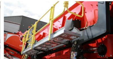
Hydraulically folding maintenance platforms
