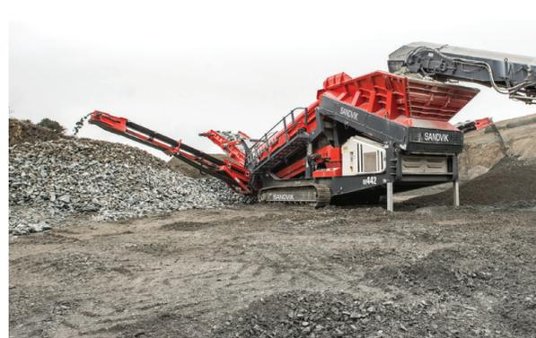
Ability to configure with punch plate, grizzly fingers, bofar bars, mesh or cascade fingers
