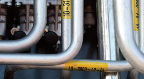
Steel pipework for better heat dissipation
